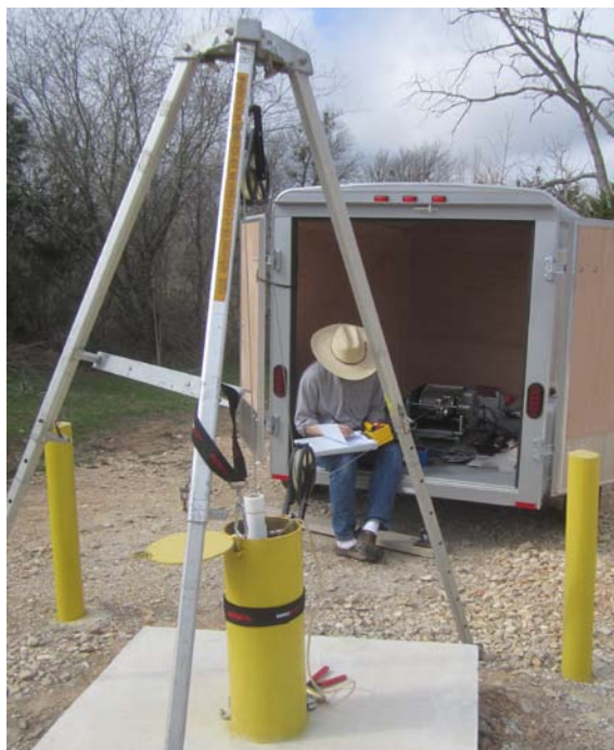
Photograph of the wellhead of the completed Antioch multiport monitor well during a sampling and water-level measurement event.
