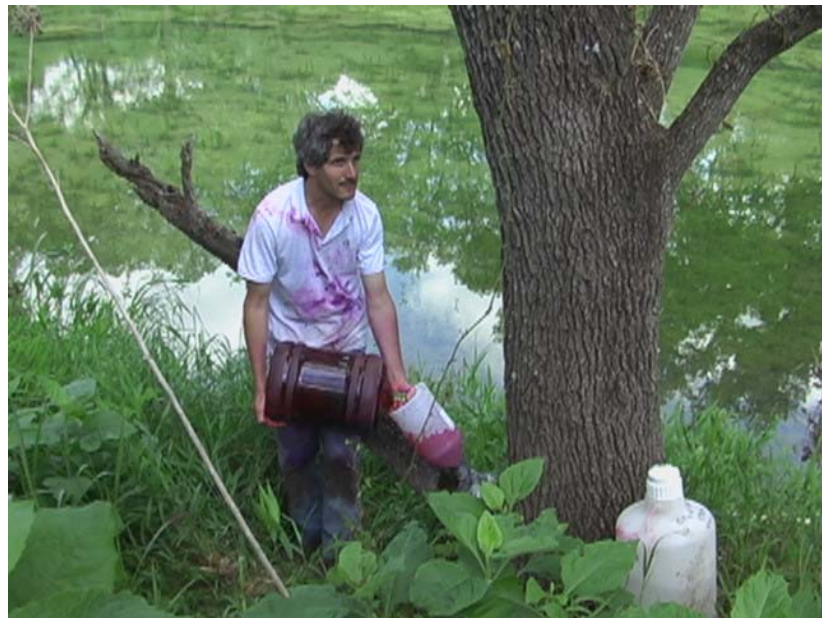
Figure 1: Mark Saunders (COA) injecting eosine dye into a PVC pipe inserted into Cripple Crawfish Cave on Onion Creek.
