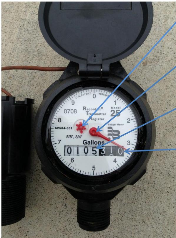
**Low Flow indicator:** Will rotate with very low flow through meter; can be used to detect small leaks.
