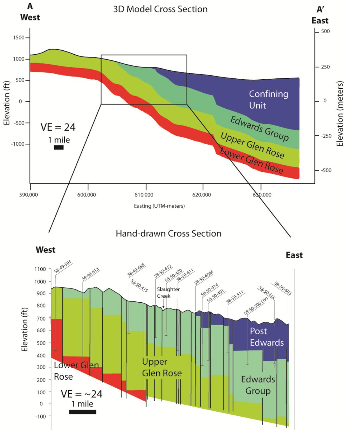
Figure 4. Two cross sections illustrating the study area geometry and demonstrates the accuracy of the 3D model across the study area. The top cross section was derived from the 3D model, and the bottom section was hand drawn based on 14 boreholes. The location of the cross section A-A' is located on Figure 3.
