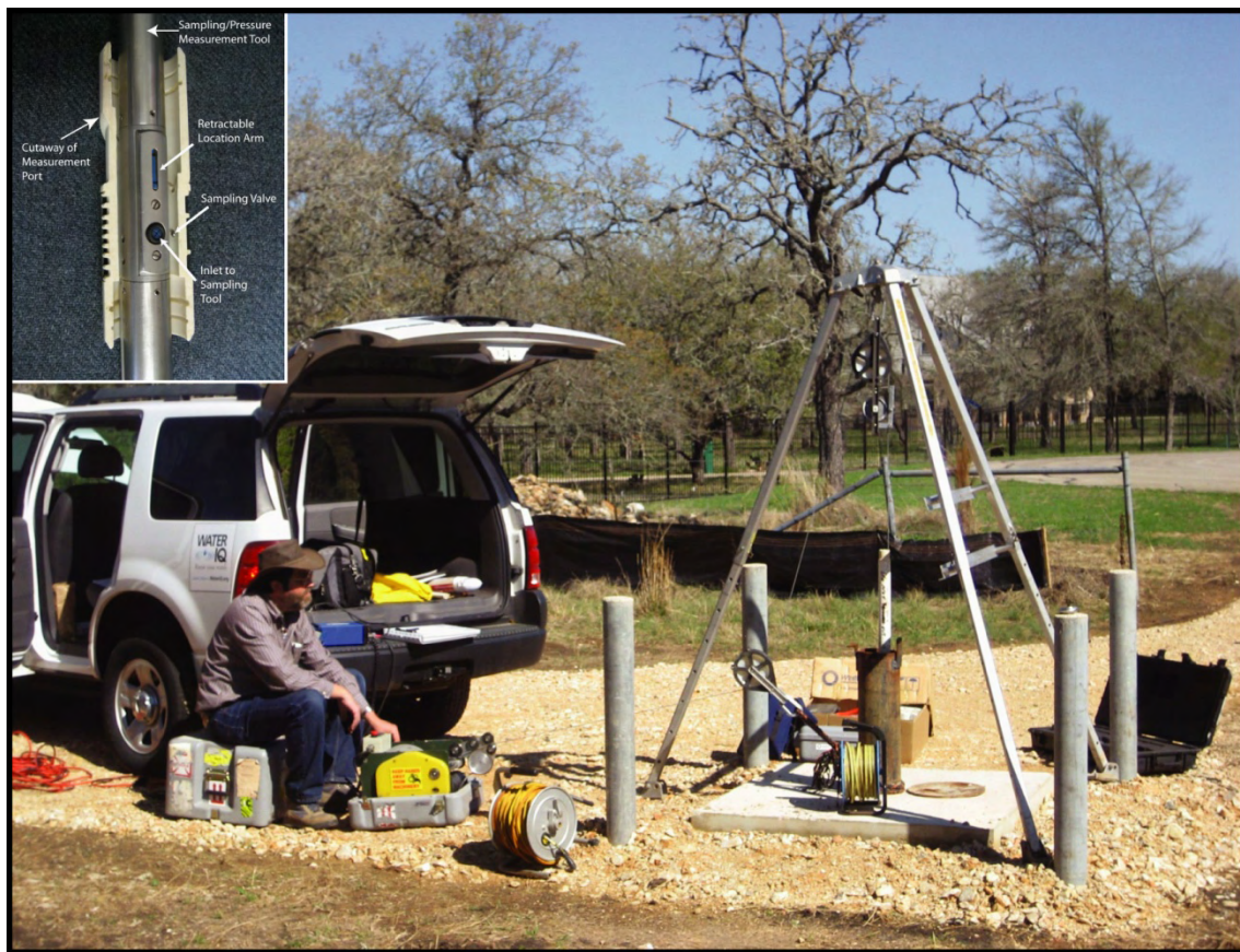
Figure 2. Picture showing data collection at the Ruby Ranch Multiport well. The wireline tool is lowered to each zone where it can measure a pressure and take a sample. Inset picture shows the sampling tool in a cut away of the casing.
