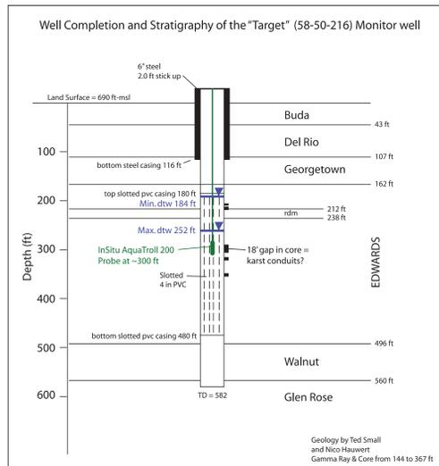
The well fully-penetrates the Edwards Aquifer. Core was taken from the well and gaps in the core could correspond to karst voids.
