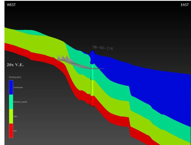
Oblique view of the geologic cross section (west to east) through the Target Well. Cross section from regional model. March 2009 potentiometric surface is denoted as gray shading.
