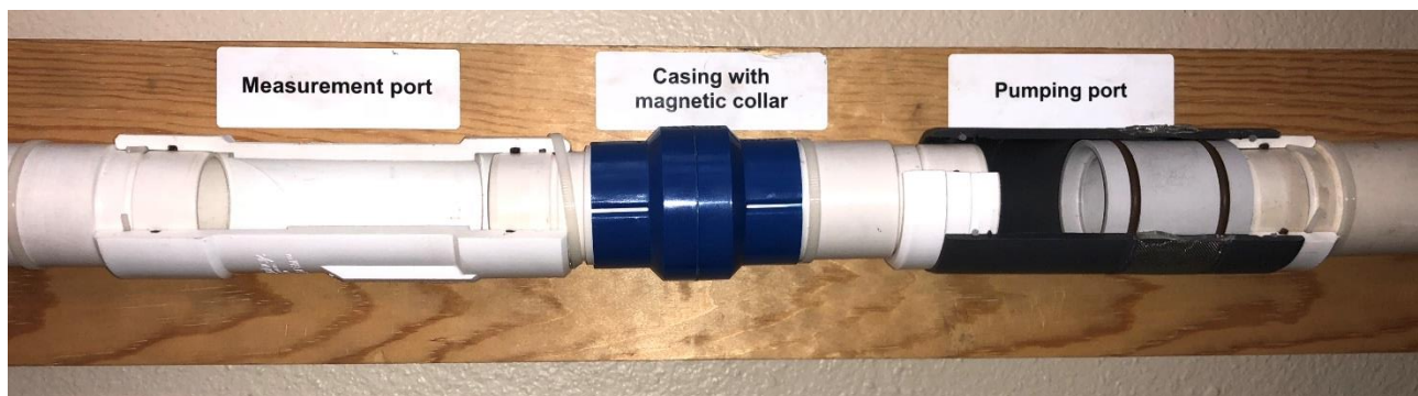
Figure 2. Cut-away model of the measurement and pumping ports, magnetic collar, and section of casing of a typical multiport monitoring zone. Not shown are hydraulic packers that are inflated in
