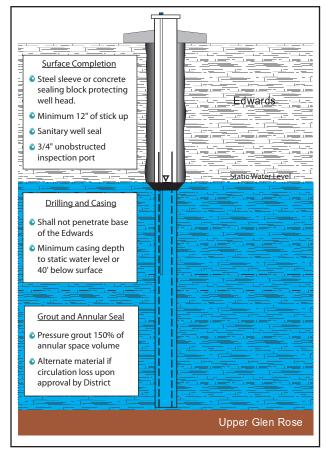
Modern wells are drilled by drilling rigs using threaded pipe and an auger. Hydrogeologists familiar local aquifer characteristics can pinpoint optimal well depths that provide the best quality and quantity of water. Since 1991, wells within the District must comply with well construction standards that have been established to protect well owners and groundwater users alike.
