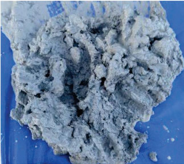
Figure 11. Photo of Del Rio Clay sample recovered from the Garrison Park Well borehole.
