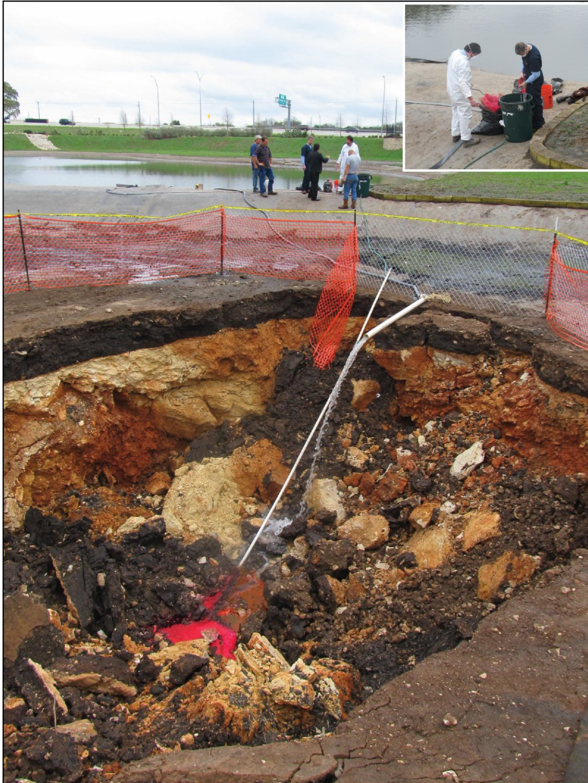
Figure 7. Phloxine B dye injection at the Arbor Trails Sinkhole. Dye was injected on February 3, 2012, at about 13:00. A mass of 16.27 lbs (7,382g) was mixed with water and then gravity injected via a hose using storm water from an adjacent pond.
