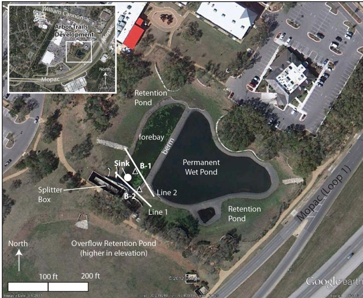
Figure 4. Detailed site map with key elements of the stormwater retention pond (SWRP), sinkhole location, and 2012 geophysics and boreholes.
