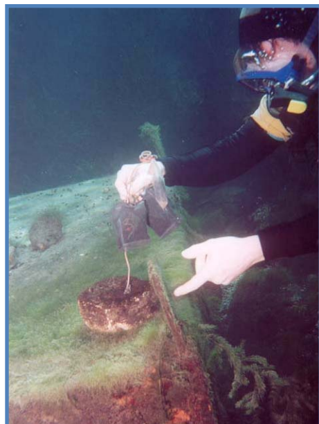
Figure 6: BSEACD staff Hydrogeologist Brian Hunt changes charcoal packets (receptors) at San Marcos Springs. San Marcos Springs are a collection of springs beneath Spring Lake, with depths up to 25 feet requiring scuba equipment to retrieve samples. Photograph taken by Brian Smith.
