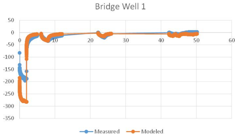
Figure 6. Comparison of measured to modeled drawdowns (in feet) for the Bridges 1 well.
