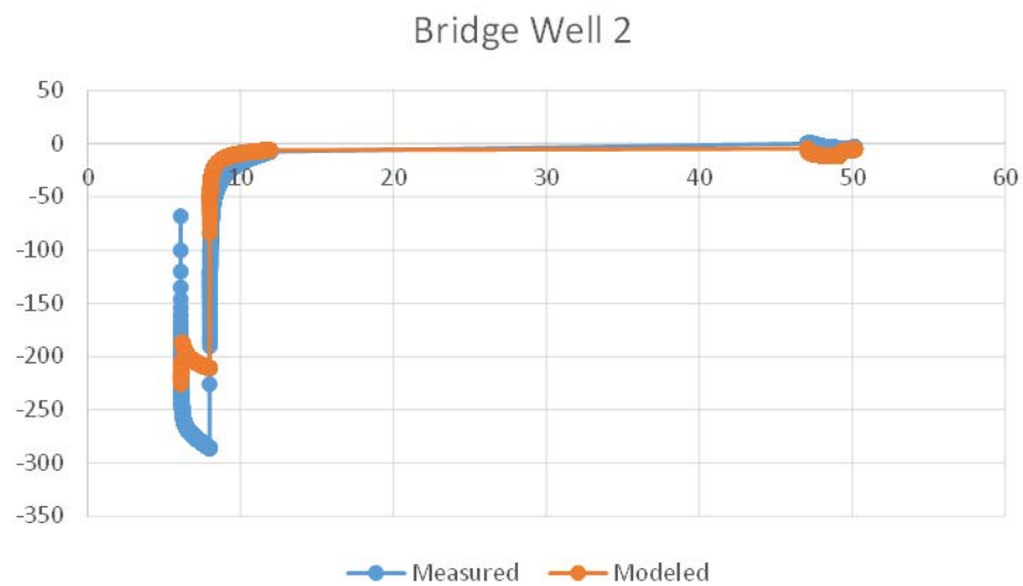
Figure 7. Comparison of measured to modeled drawdowns (in feet) for the Bridges 2 well.
