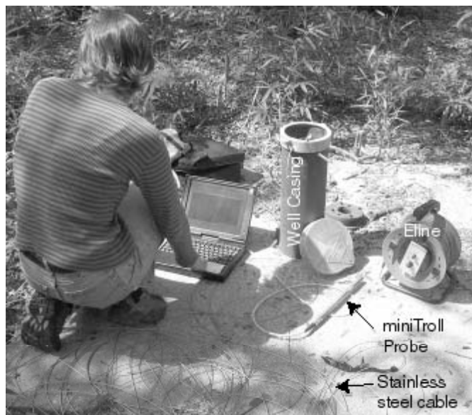
Figure 2. Stefani Campbell down-loads data from the Insitu miniTroll probe onto the laptop at the Sunset Valley (58-50-417) well.
