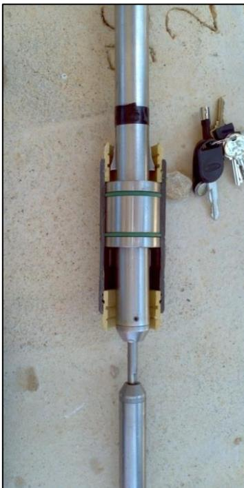
**Figure 9. Picture of the pumping port and tool implemented for opening and closing. Sleeve is in open position with the open-close tool in a position to close the sleeve.**
