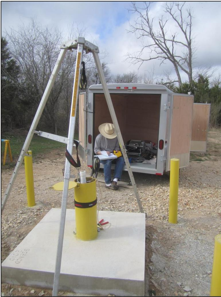
**Figure 7. Photograph showing data collection from the multiport well. The wireline tool is lowered by the winch in the trailer. Control of the sampling tool and display of data are done electronically.**
