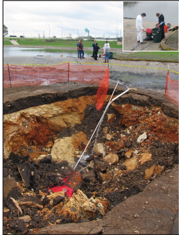
Figure 8. Phloxine B dye injection at Arbor Trails sinkhole. Dye was injected on February 3, 2012. A mass of about 7 kg (16 lbs) was mixed in a trash can and then gravity injected via a hose and polyvinyl chloride (PVC) pipe using water from an adjacent wet pond.
