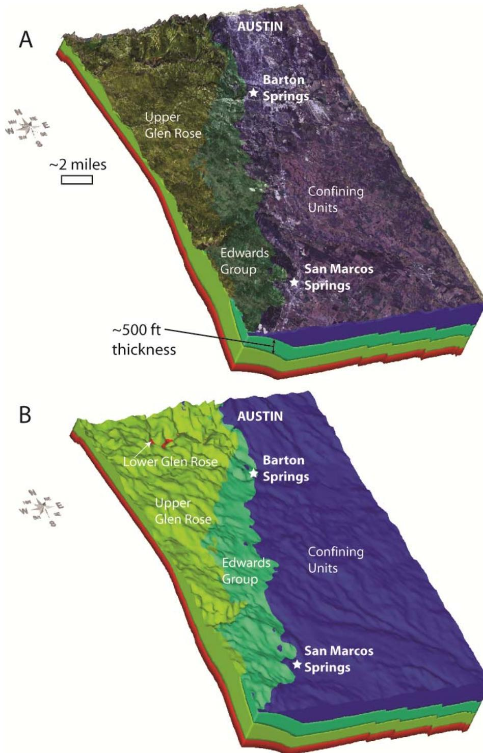
Figure 5. (A) Screen capture of the model from an elevated perspective to the southwest with satellite image overlaid and 50% transparent. (B) Same image as top but with satellite overlay turned off and features labeled.
