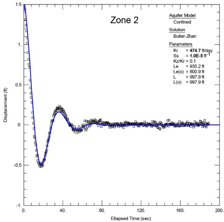
**Figure 20.** Example slug test analyses and curves from Aqtesolv. Top figure represents overdamped water-level response and solutions include the KGS and Bouwer-Rice solutions that produced similar values. The lower figure represents underdamped (high permeability) water-level response and the Butler-Zhan solution to estimate permeability.
