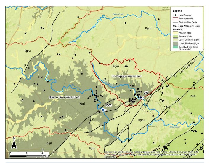
**Figure 2.** Geologic map of the region around Jacob's Well (JW) and Pleasant Valley Spring (PVS) and their respective watersheds. The area outlined in dark red is upgradient of Jacob's Well and is defined in this report as the Dry Cypress Creek watershed (31 square miles). The Lower Glen Rose carbonates are exposed in the dark green area and contain the majority of known karst (recharge) features in the Trinity Group units.
