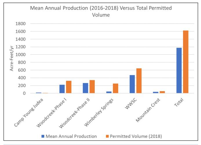
**Figure A-5:** Comparison of permitted annual volume versus average reported actual pumping (2016 through 2018) for large permit holders with wells in one of the three delineated Jacob's Well areas of influence. Total permitted volume is significantly larger than average reported pumping for most of the large permits.
