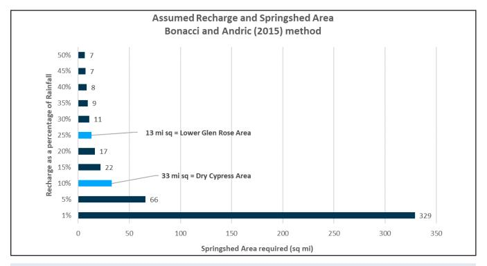
**Figure 9.** Results of assumed recharge as a percentage of precipitation and the calculated springshed area. The area of Dry Cypress Creek watershed is about 31 square miles, or about 10 percent of precipitation. The Lower Glen Rose has an area within Dry Cypress Creek watershed of 12.1 square miles, or about 25 percent of precipitation.
