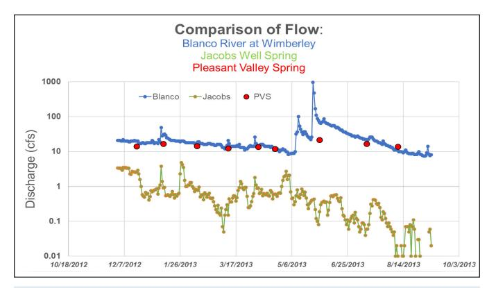
**Figure 8.** Springflows and Blanco River (at RR12) hydrograph. Note the increased Pleasant Valley Spring springflow and Blanco River response in May to June 2013, while Jacob's Well had no corresponding response. Source data from USGS (2017a, 2017b) and Marcus Gary (unpublished data).
