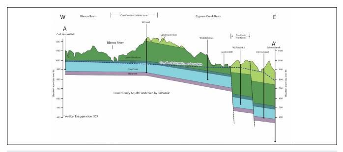
Figure 6. Structural cross section and October 2018 potentiometric surface. Figure from Broun and Watson (2018). Line of cross section shown in Figure 7.
