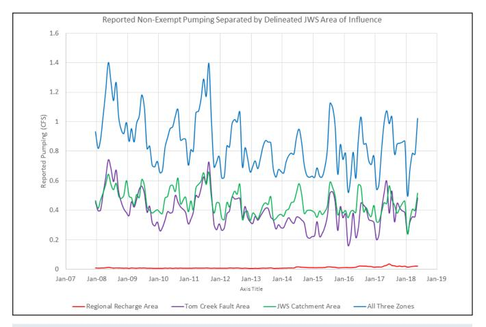
**Figure 19:** District reported non-exempt pumping in each delineated Jacob's Well area of influence. Distinctive peaks in pumping coincide with the summer months. Tom Creek Fault Area production is estimated. CFS = cubic feet per second, JWS = Jacob's Well Spring
