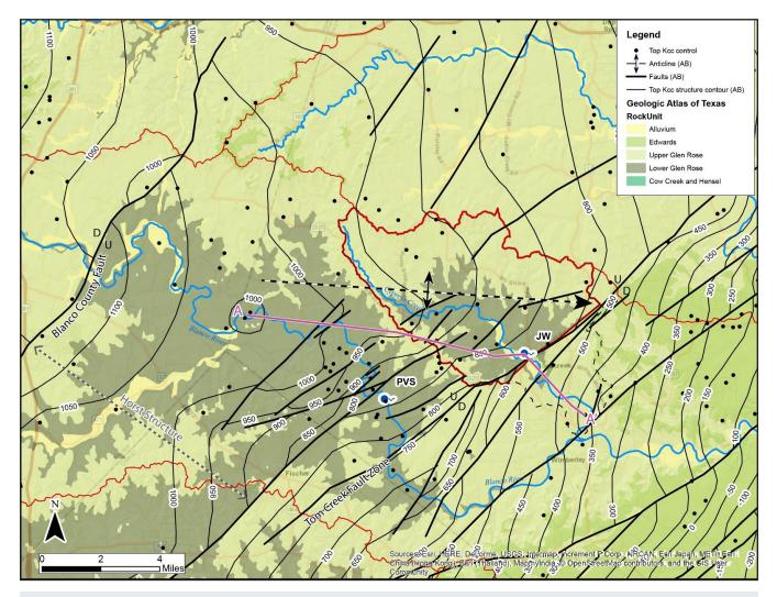
**Figure 5.** Structure contour map of the top of the Cow Creek (contours in feet above mean sea level). Contours, control, and faults from Al Broun (unpublished data). Figure modified from Wierman and others, 2010. Cross section A to A' is shown in Figure 6.
