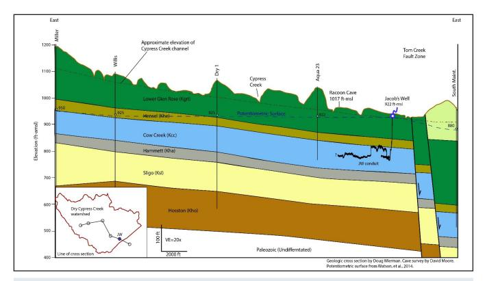
Figure 4. Geologic cross section through Dry Cypress Creek watershed. The potentiometric surface is for the Middle Trinity Aquifer.
