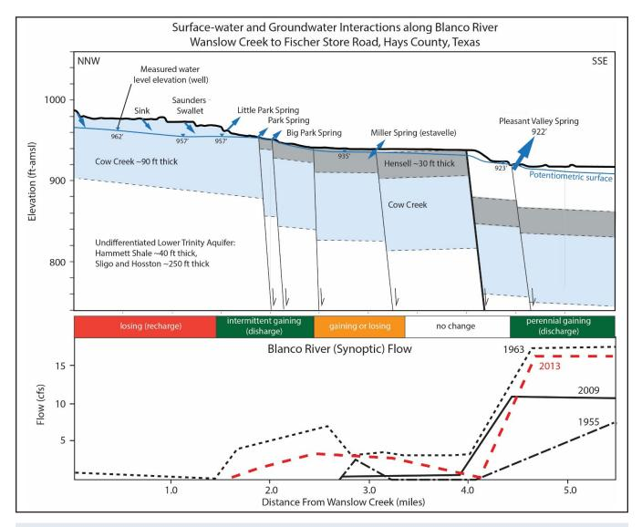
**Figure 17.** Detailed cross section and flow rate graph show the surface-water/groundwater interaction of the spring reach of the Blanco River from Gary and others, 2013). Synoptic Blanco River flows indicates flows that occurred within a short period of time, generally less than a few weeks. Synpotic flow events were made during low-flow conditions.
