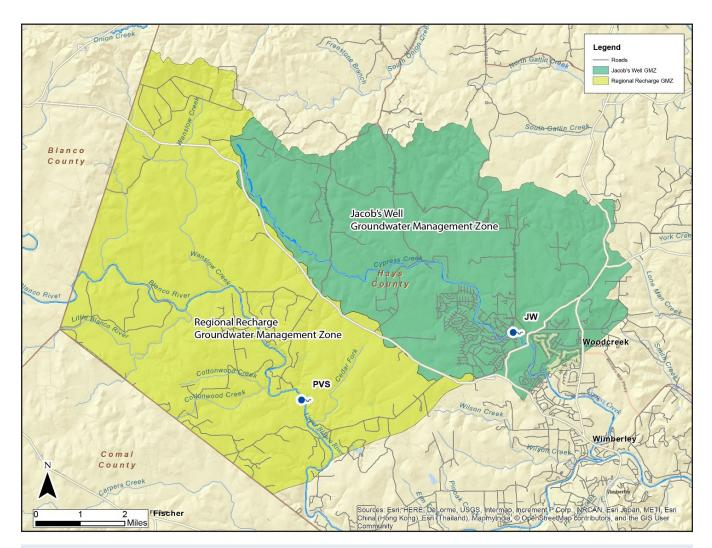
**Figure ES-1.** Areas of hydrologic influence to Jacob's Well shown in hatched areas. Potential groundwater management zones are shaded green and yellow. The area of the Jacob's Well Groundwater Management Zone is 34 square miles and the area of the Regional Recharge Groundwater Management Zone is 56 square miles.
