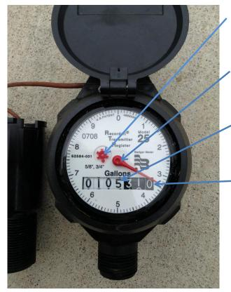
**Low Flow indicator**: Will rotate with very low flow through meter; can be used to detect small leaks.
