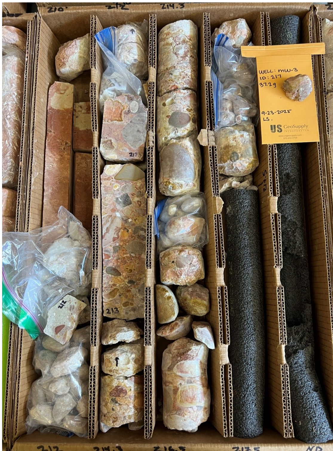
Figure 3.4 Lower pebble to cobble conglomerate interval at the base of the Sycamore Sand (Hosston Formation) of MW#3. Note the tight cementation and very poorly sorted clasts. The bottom of the core is at 217.5 ft, where the black foam spacer begins.
