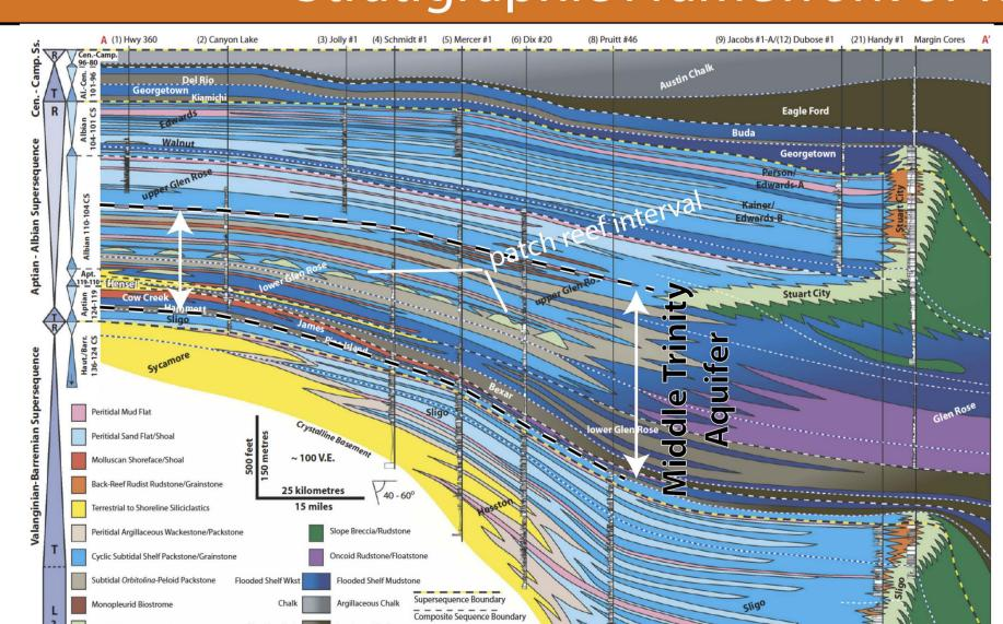
The Middle Trinity Aquifer is composed of (from stratigraphically lower to highest) the Cow Creek, Hensel, and the Lower Glen Rose Formations. It is the primary aquifer in the Trinity Aquifer system for water-supply needs in the Hill
