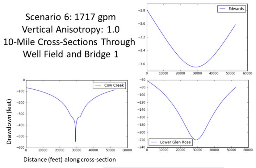
Figure A-6. Drawdown profiles for Scenario 6 across a 10-mile cross-section through the EP well field.
