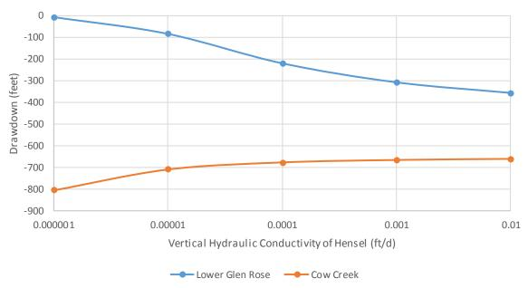
Figure 13. Sensitivity of Cow Creek and lower Glen Rose drawdown to the vertical hydraulic conductivity of the Hensel. Assumes pumping in the EP well field of 2.47 million gallons per day. Drawdowns after 50 years shown for Bridges 1 well.
