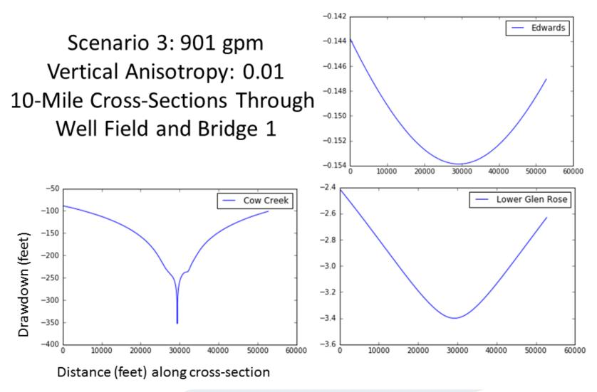
Figure A-3. Drawdown profiles for Scenario 3 across a 10-mile cross-section through the EP well field.
