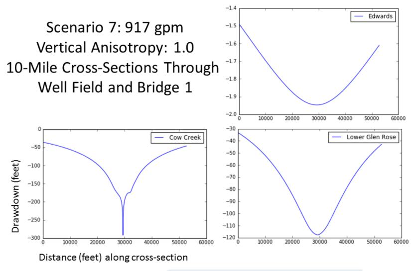
Figure A-7. Drawdown profiles for Scenario 7 across a 10-mile cross-section through the EP well field.
