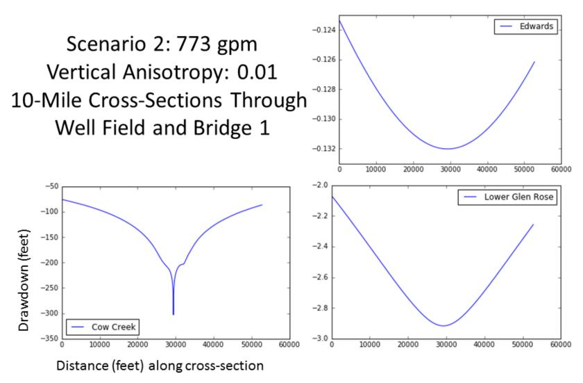
Figure A-2. Drawdown profiles for Scenario 2 across a 10-mile cross-section through the EP well field.
