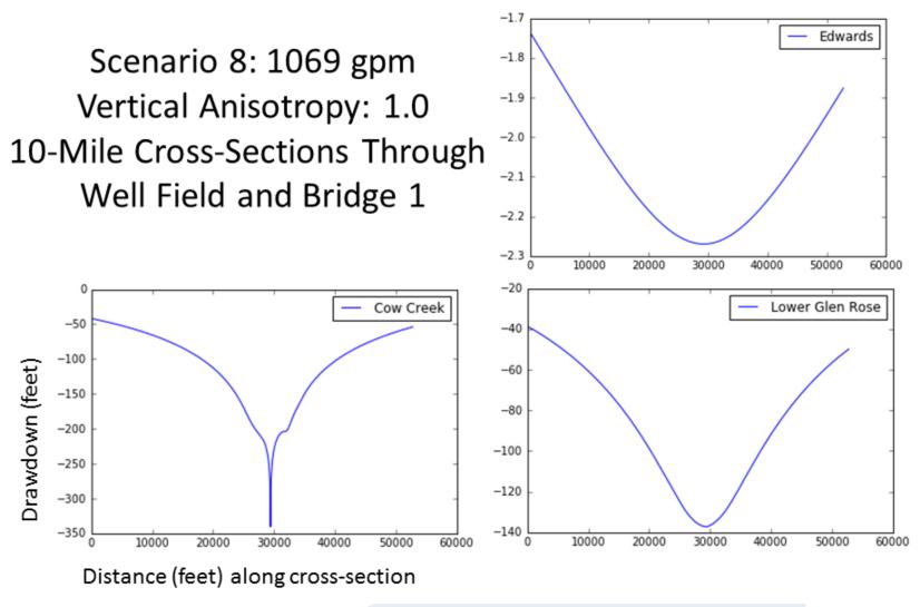
Figure A-8. Drawdown profiles for Scenario 8 across a 10-mile cross-section through the EP well field.
