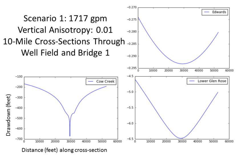
Figure A-1. Drawdown profiles for Scenario 1 across a 10-mile cross-section through the EP well field.
